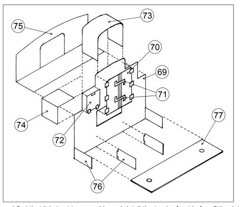
4. I find that it is best to assemble and detail the tender front before fitting into place. Take the front bulkhead (part 69) and fit the fireman's tunnel doors (part 70). Then solder the door catch detail overlays (parts 71) over the raised outlines. Fit the tool box door detail overlays (parts 72) slightly inboard of the corner edges.
