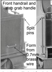
The handrails are formed from 0.7mm brass wire. Only the front handrails were supported by any form of handrail knob and even if you normally use handrail knobs I would recommend using the split pins as they better represent the prototype supports.
