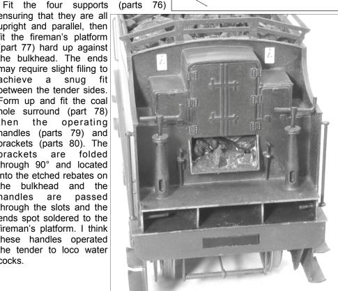
5. Fit the rear coal space bulkhead (part 81) into the slots on the tender top. Fit the reinforcing angles (parts 82) locating into the slots on the bulkhead and fit the rivet detail overlays (parts 83) into each corner and against the reinforcing angles.
