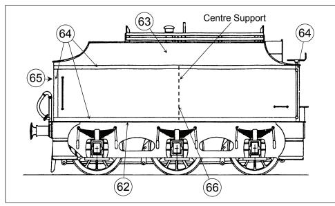
8. We are now down to the detailing and fitting of the castings. I leave these to this stage so that they wont get damaged with the repeated handling of the main construction. These parts can be fitted in whatever order takes your fancy but I tend to fit the parts that require higher temperature soldering first. First the handrails then the lamp brackets and then the coupling. Then I fit the castings.
