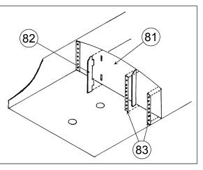
across the tender back and both bulkheads. The strips that run across will need their ends trimming back slightly to be a snug fit between the side beading. Place a spot of solder onto the top surface at the beading joints and then blend in with a file.
