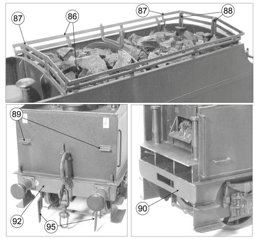
6. Fold the tender back steps (parts 89) through  $90^{\circ}$  and solder into half etched rebates. Fit the front drag beam (part 90) locating into the half etched grove on the underside of the footplate. Emboss bolt heads on the tender frames (parts 91) and fit into slots on footplate underside so that the end is hard against the front buffer beam. Fit the rear buffer beam (part 92) tight up against the ends of the frames.
