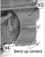
Fold a set in each guard iron (parts 95) using the etched marks as guides. Solder into the slots on the underside of the footplate. Tweak the folds on the guard irons with long nosed pliers to achieve a distance of 32mm (track gauge) apart and reinforce the fold lines with solder.
