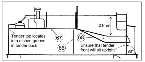
Now pull coal space hopper upwards and tack solder into place, adjusting the coal space to get the best fit as you go. Once happy with the shape and fit solder solid, filling all gaps with solder. Now check the front end to ensure that the tender front (part 69) will sit upright and square. If necessary file back the front of the coal space using a sharp flat file to achieve this.
